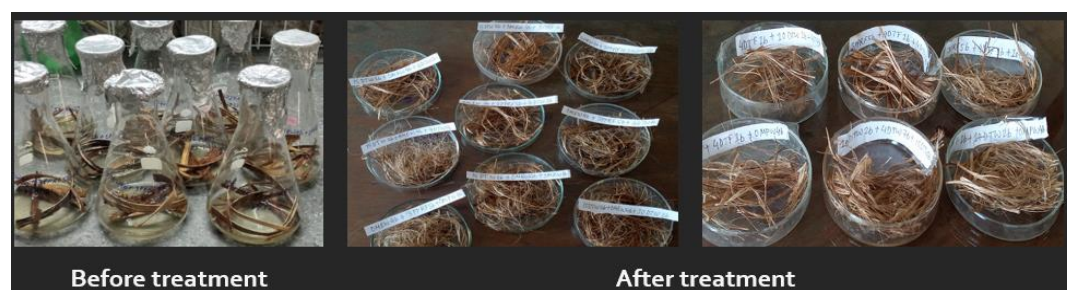
Fig. 1. Treatment of preserved CVL-1 dry fiber with the selected microbial broth of three combinations with water
