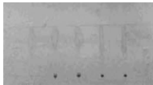
Fig. 14 TLC of lubricating oils from biodiesel-fuelled engine using rhodamine-B as revealing agent
