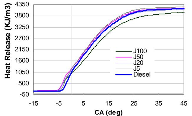
Figure 14f: Cumulative heat release vs. crank angle diagram for 100% rated engine Load
