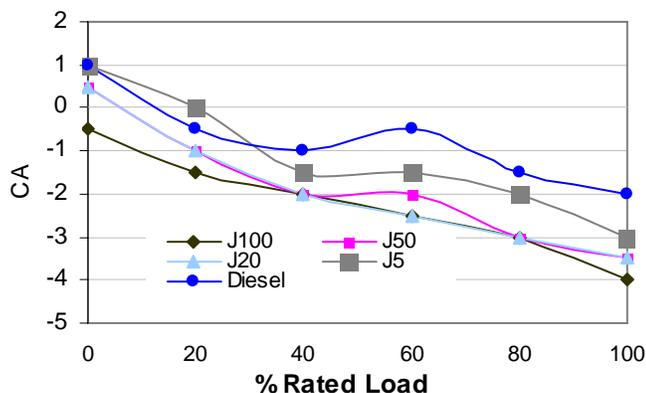
Figure 17b: Crank angle for maximum rate of pressure rise for different engine loads
