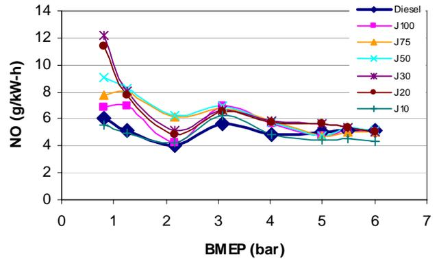
Figure 11: Comparison of NO emissions of Jatropha oil blend fuelled engines
