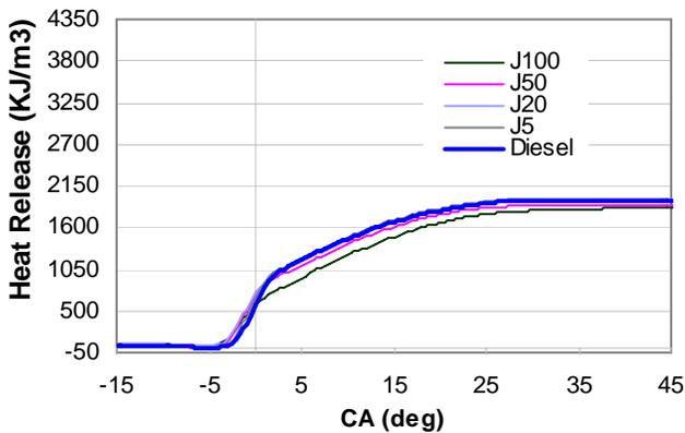
Figure 14c: Cumulative heat release vs. crank angle diagram for 40% rated engine Load
