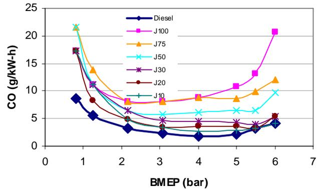
Figure 6: Comparison of CO emissions of Jatropha oil blend fuelled engines
