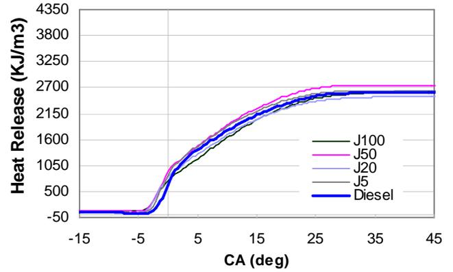
Figure 14d: Cumulative heat release vs. crank angle diagram for 60% rated engine Load
