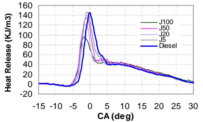
Figure 13d: Instantaneous Heat release vs. crank angle diagram for 60% rated engine Load
