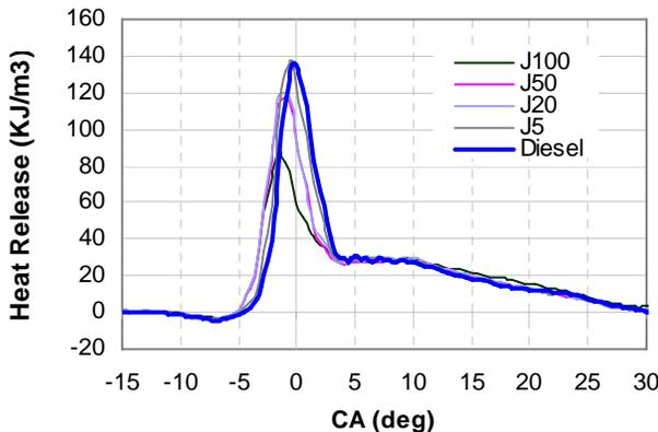
Figure 13c: Instantaneous Heat release vs. crank angle diagram for 40% rated engine Load
