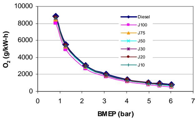
Figure 10: Comparison of oxygen content in exhaust gas of Jatropha oil blend fuelled engines
