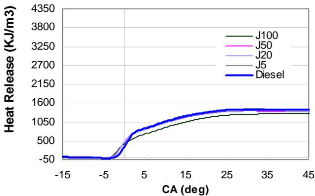
Figure 14b: Cumulative heat release vs. crank angle diagram for 20% rated engine Load
