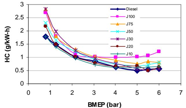
Figure 7: Comparison of HC emissions of Jatropha oil blend fuelled engines
