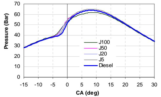
Figure 12e: Pressure–crank angle diagram for 80% rated engine Load
