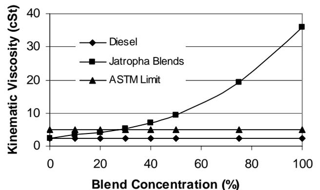
Figure 2: Viscosity of various Jatropa oil blends at 40°C
