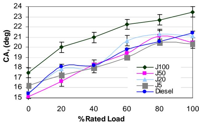
Figure 15c: Crank angle for 90% mass fraction burn
