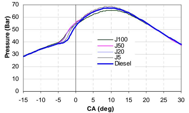
Figure 12f: Pressure–crank angle diagram for 100% rated engine Load
