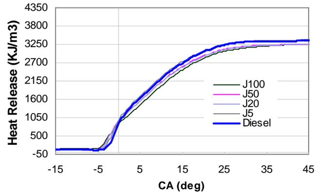
Figure 14e: Cumulative heat release vs. crank angle diagram for 80% rated engine Load
