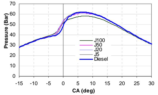
Figure 12d: Pressure–crank angle diagram for 60% rated engine Load
