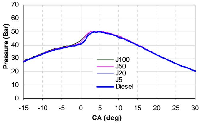
Figure 12a: Pressure–crank angle diagram for 0% rated engine Load
