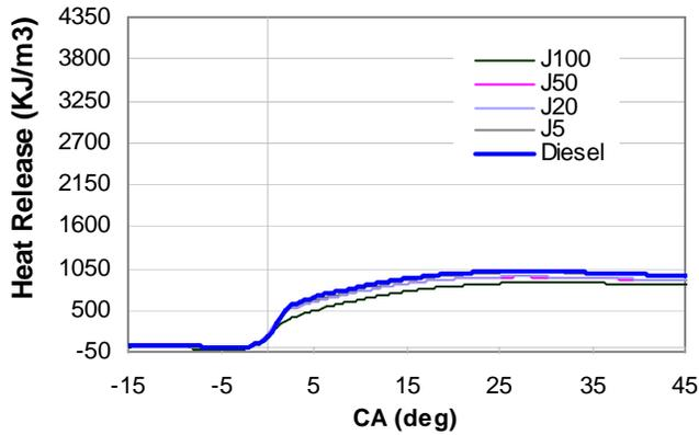
Figure 14a: Cumulative heat release vs. crank angle diagram for 0% rated engine Load
