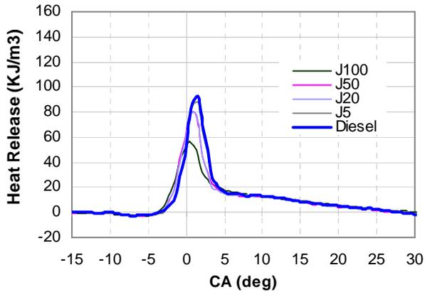
Figure 13a: Instantaneous Heat release vs. crank angle diagram for 0% rated engine Load
