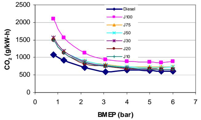
Figure 5: Comparison of CO<sub>2</sub> emissions of Jatropha oil blend fuelled engines
