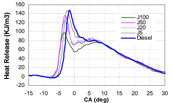
Figure 13f: Instantaneous Heat release vs. crank angle diagram for 100% rated engine Load
