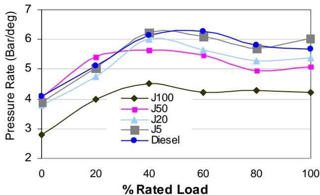
Figure 17a: Maximum rate of pressure rise for different engine loads
