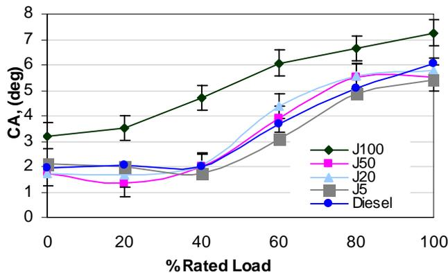
Figure 15b: Crank angle for 50% mass fraction burn
