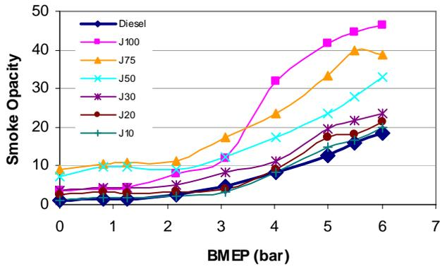
Figure 8: Comparison of smoke opacity of Jatropha oil blend fuelled engines
