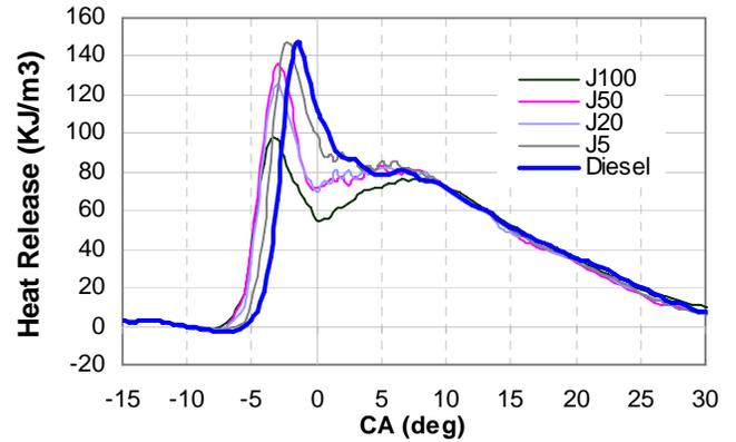
Figure 13e: Instantaneous Heat release vs. crank angle diagram for 80% rated engine Load
