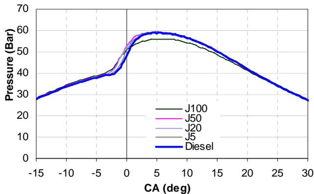
Figure 12c: Pressure–crank angle diagram for 40% rated engine Load
