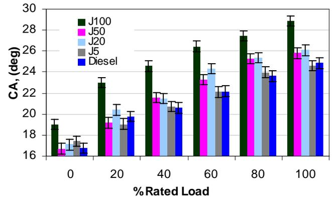
Figure 18: Combustion Duration for unheated Jatropa oil and blends vis-à-vis mineral diesel
