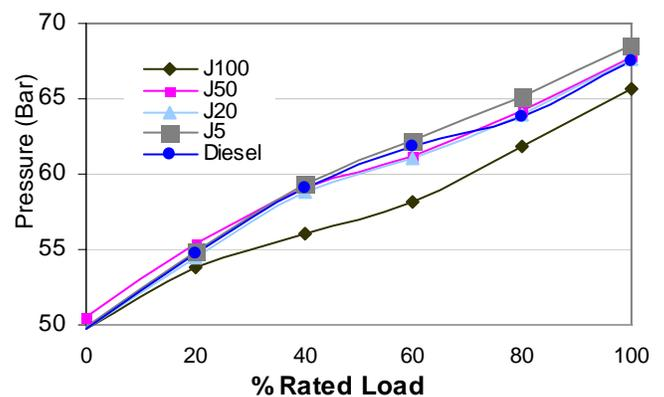
Figure 16a: Maximum in-cylinder pressure for different engine loads
