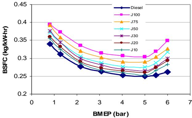
Figure 3: Comparison of bsfc of Jatropha oil blend fuelled engines
