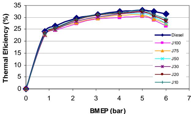
Figure 4: Comparison of thermal Efficiency of Jatropha
