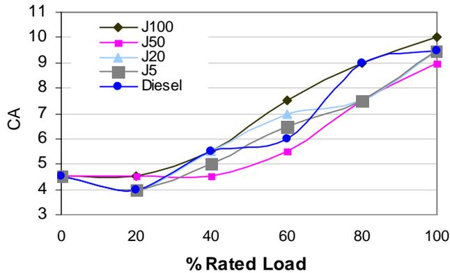
Figure 16b: Crank Angle at maximum in-cylinder pressure for different engine loads
