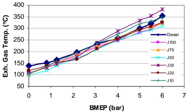
Figure 9: Comparison of exhaust gas temperature of Jatropha oil blend fuelled engines
