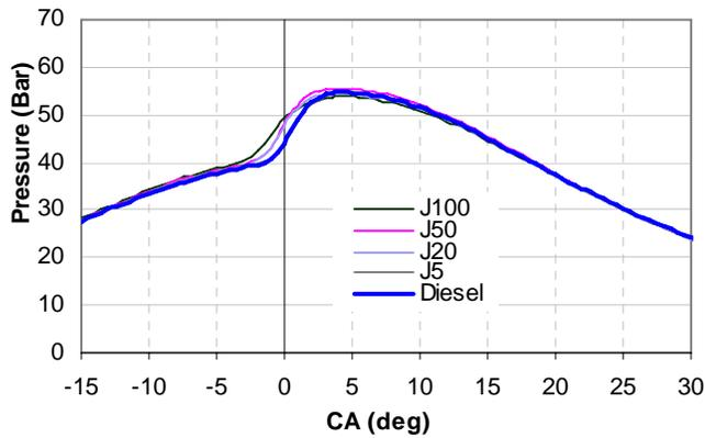
Figure 12b: Pressure–crank angle diagram for 20% rated engine Load
