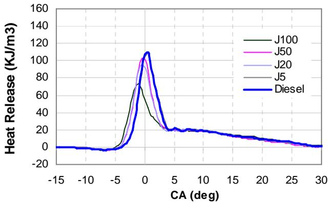
Figure 13b: Instantaneous Heat release vs. crank angle diagram for 20% rated engine Load
