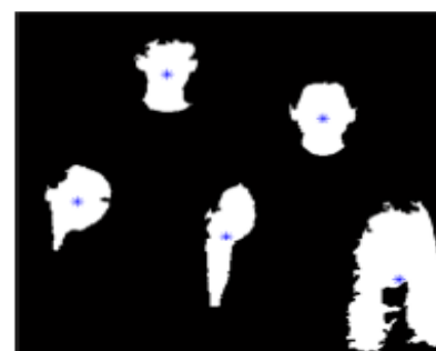
Fig. 6 - Result after calculating centroid
