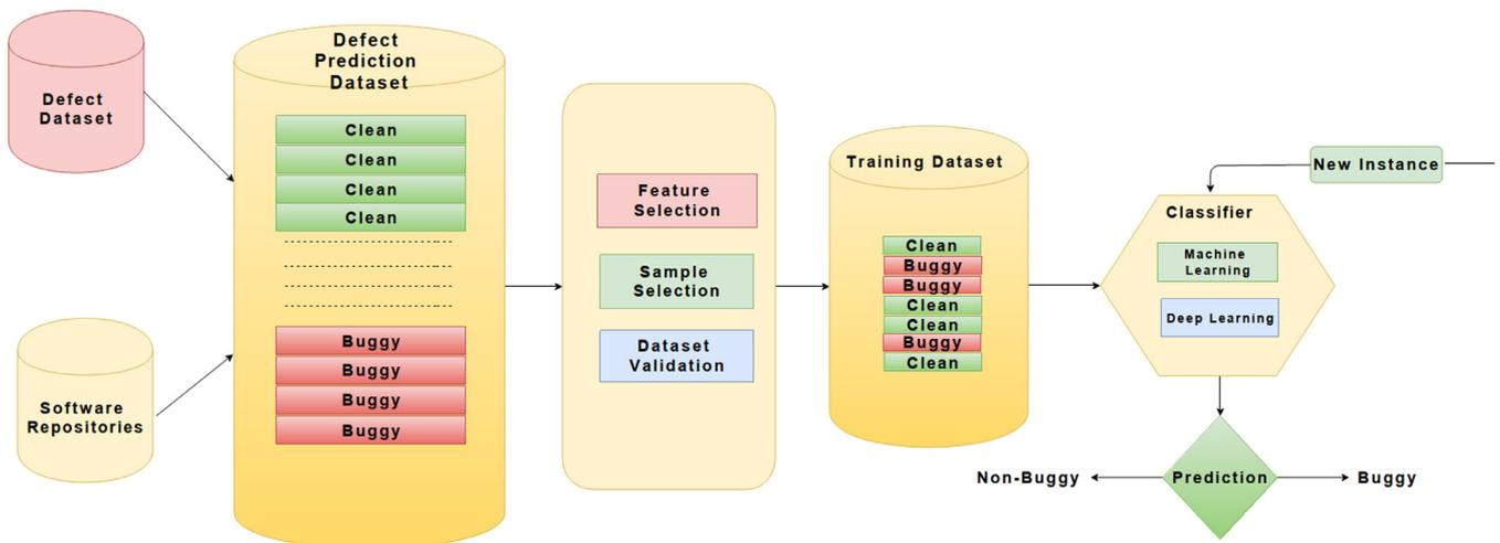
Fig. 5. Software Defect Prediction — general approach.
