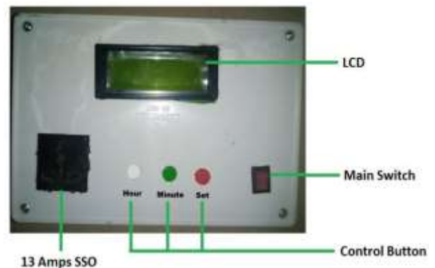
Figure 13. Constructed Arduino Timer Socket Unpowered.
