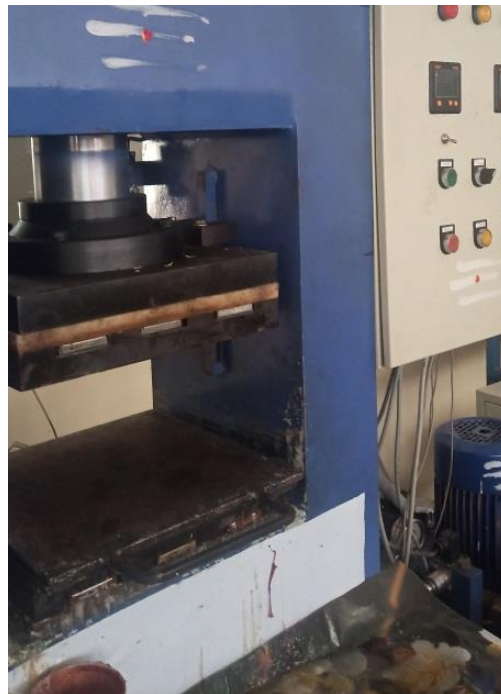
Fig. 2. Compression molding machine used for composite fabrication.
