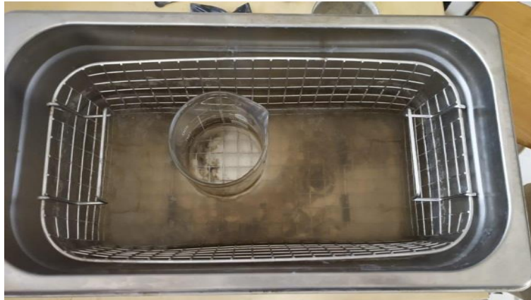
Fig. 1. Ultrasonication of epoxy with nano-filler
