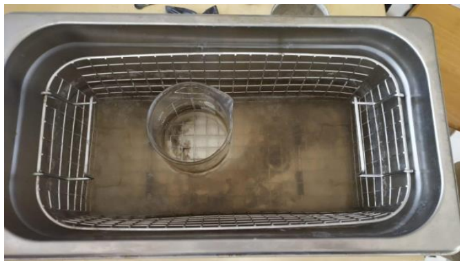
Fig. 1. Ultrasonication of epoxy with nano-filler.
