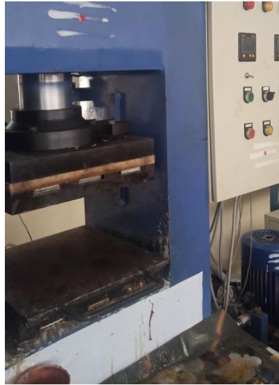
Fig. 2. Compression molding machine used for composite fabrication.
