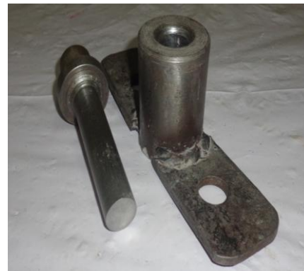
Fig. 2 Die set to fabricate cylindrical preform
