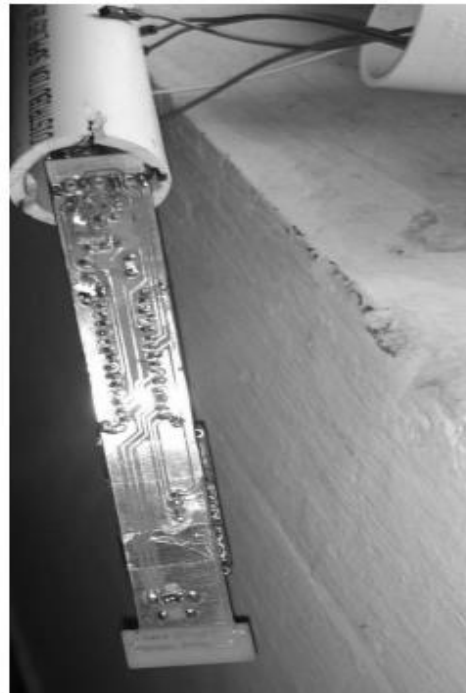
Fig 10.2: Back side of printed circuit board with components for Guidance System for Blinds
