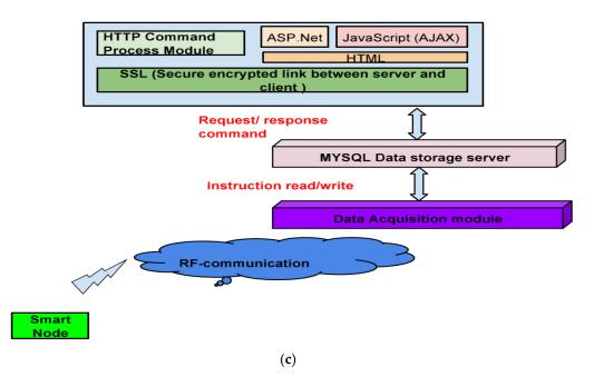
**Figure 2.** Detailed workflow of the system. (**a**) CP Plus 850 tvl analog camera; (**b**) customized hardware in which the proposed research methodology is coded; and (**c**) the layered architecture of an anti-theft system for an Internet of Things (IoT)-based smart home solution.
