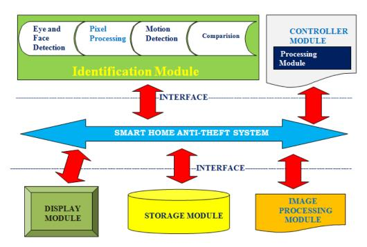
Figure 5. Communication block diagram of the smart home anti-theft system.
