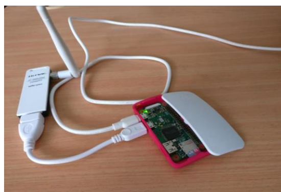
Figure 4: Raspberry pi connected with network adapter
