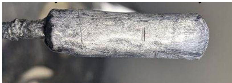
Figure S4: Dense neodymium deposit produced with chloride MSE. This deposit was produced on a W cathode subjected to 0.5 A/cm 2 current density in a 1.65 M NdCl 3 ·6H 2 O containing LiCl–KCl melt at 500 °C for 1 hour. This shows feasibility of utilizing hydrated NdCl 3 as the feedstock.
