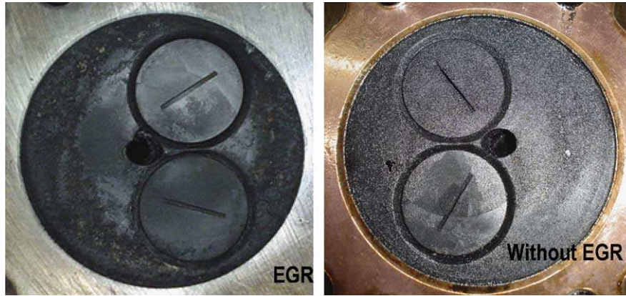
Fig. 2. Carbon deposits on the cylinder head after 96 h of engine operation.
