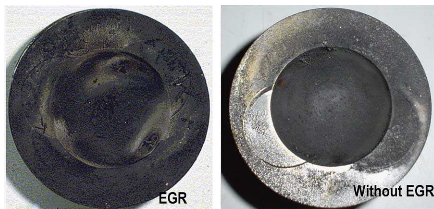
Fig. 4. Carbon deposits on the piston crown after 96 h of engine operation.
