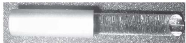
Fig. 2 (f): 70° degree Illumination Tip
