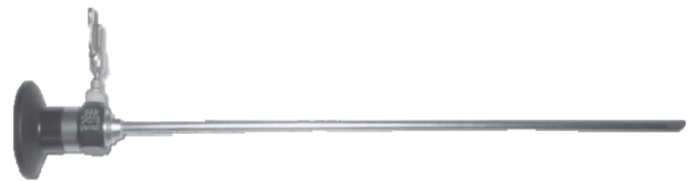
Fig. 2 (c): Typical engine endoscope
