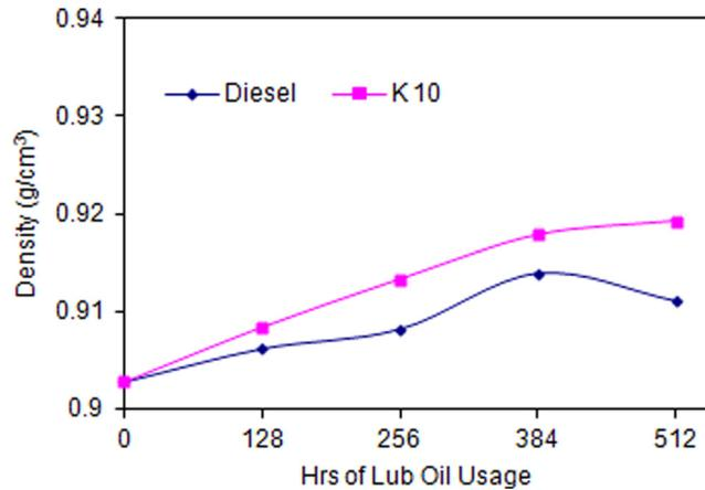
FIG. 3. Density of the lubricating oils during the endurance test.
