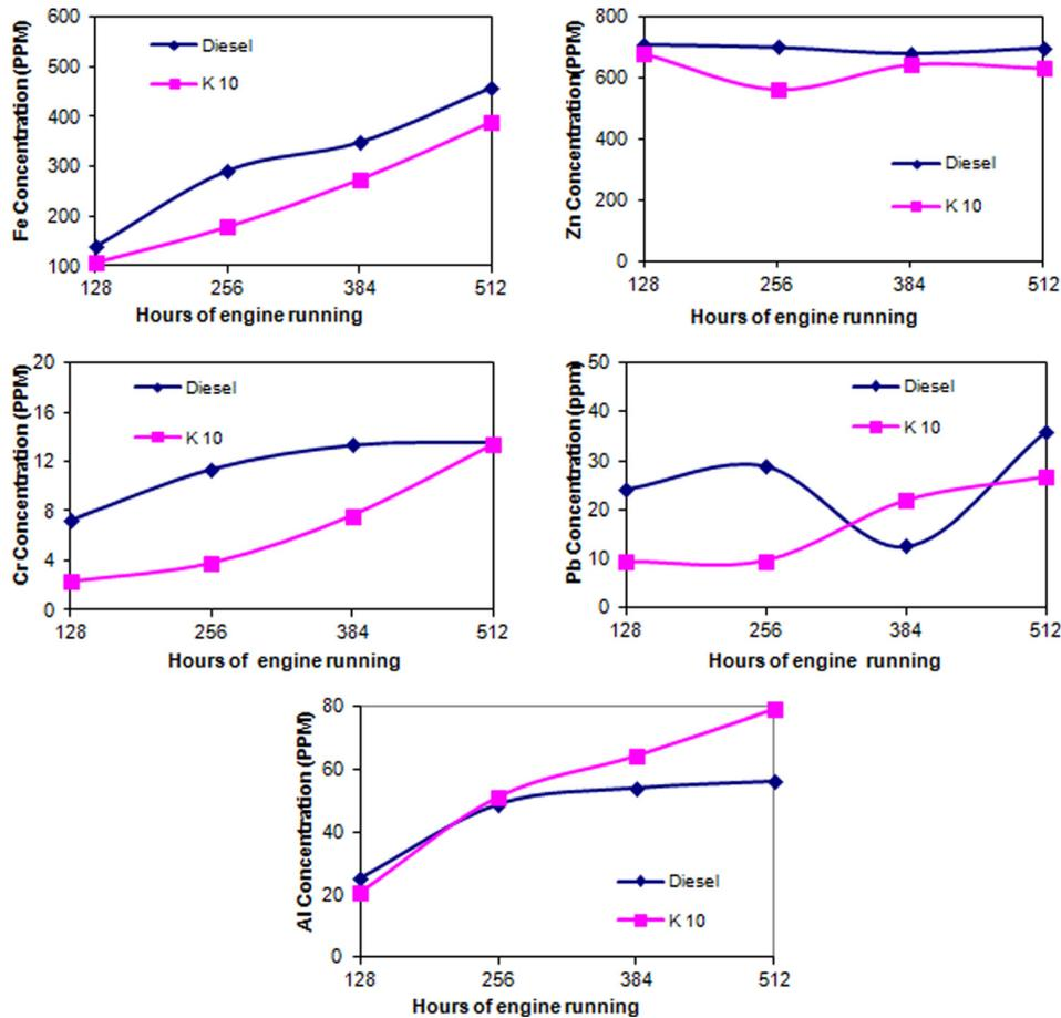
FIG. 9. Concentration of various trace metals in the lubricating oils during the endurance test.
