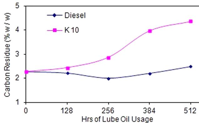
FIG. 8. Carbon residue of the lubricating oils during the endurance test.
