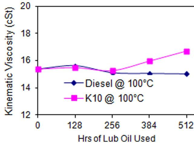
FIG. 5. Viscosity of the lubricating oils at 100 °C during the endurance test.
