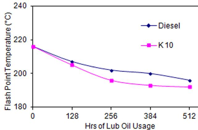
FIG. 6. Flash point of the lubricating oils during the endurance test.
