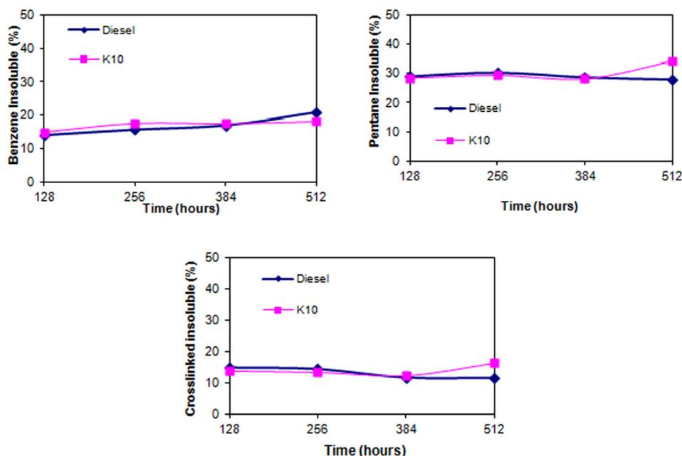
FIG. 10. (a) Benzene insoluble, (b) pentane insoluble, (c) cross-linked insoluble of the lubricating oils during the endurance test.
