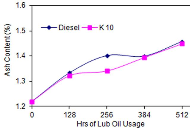
FIG. 7. Ash content of the lubricating oils during the endurance test.
