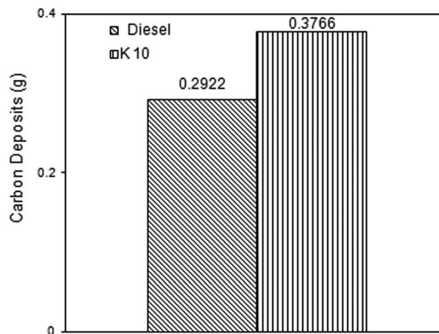
FIG. 2. Carbon deposits on the piston top after the endurance test.
