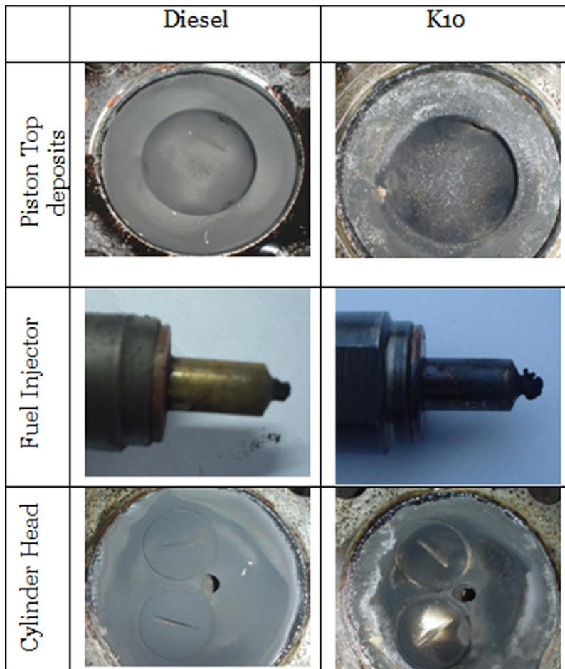
FIG. 1. Carbon deposits on piston top, injector and cylinder head after the endurance test.
