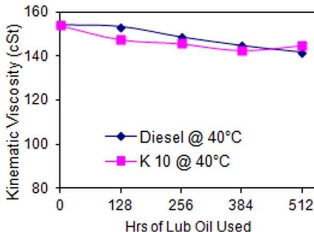
FIG. 4. Viscosity of the lubricating oils at 40°C during the endurance test.
