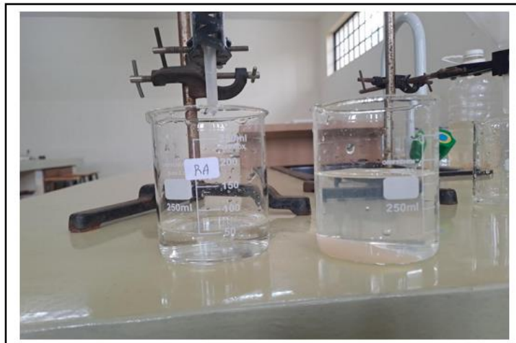
Figure 3: Flocs in the treated river water samples
