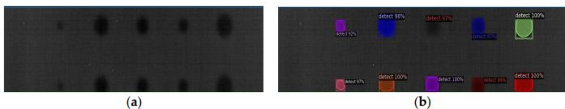
Figure 17. An example of used Method: 6(a) the original thermal image; (b) the detected image.
