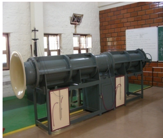
Fig. 3 Side View of Ducted Axial Fan Rig
