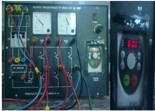
Fig.4 Variable frequency Drive for speed control
