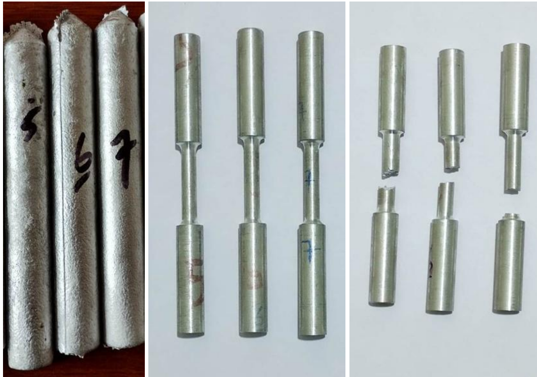
Figure 4: Casted samples, machined as per slandered and after tensile test backed samples.
