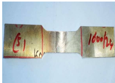
Fig 3: (b) Mechanical Test Piece for UTM
