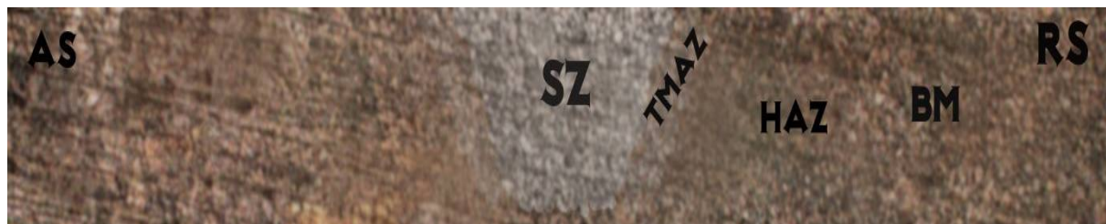
Fig 4: Macroscopic Images of the Welded Joint Showing the Evolution of FSW Zones
