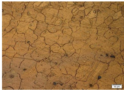
(c) Heat Affected Zone (HAZ) (1600rpm/ 24 mm/min)
