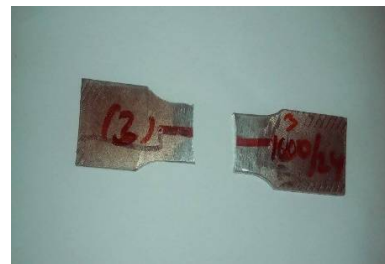
Fig 3: (c) Mechanical Test Piece after UTM
