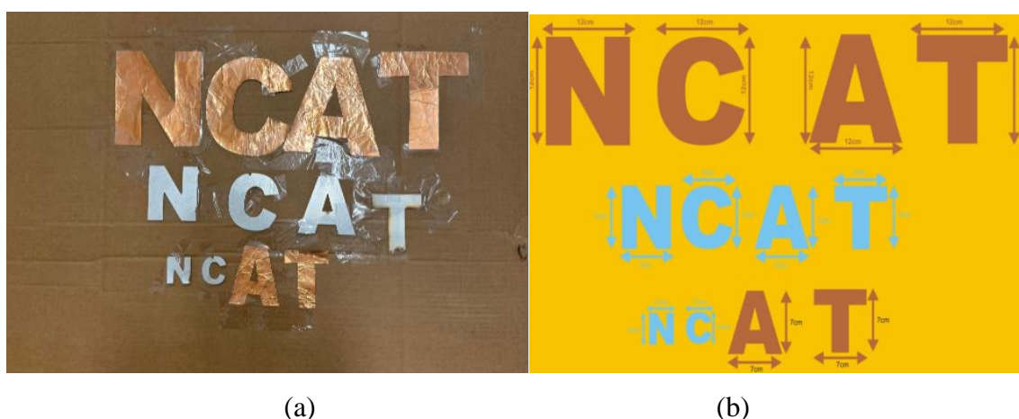
Figure 3: Alphabetical letter target (a) Physical depiction (b) Dimensions
