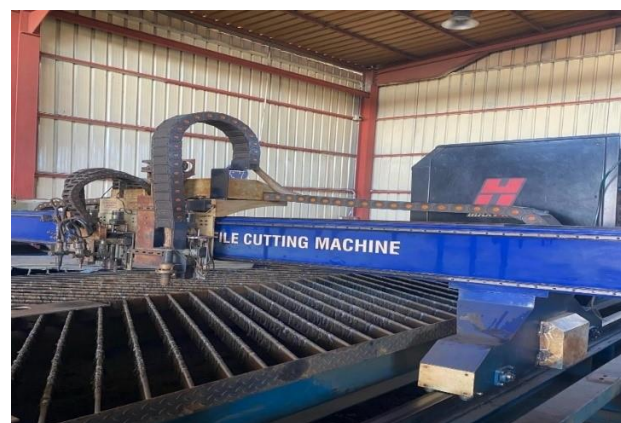
Figure 15: The plasma cutting machine and the attachment at the end of the piston
