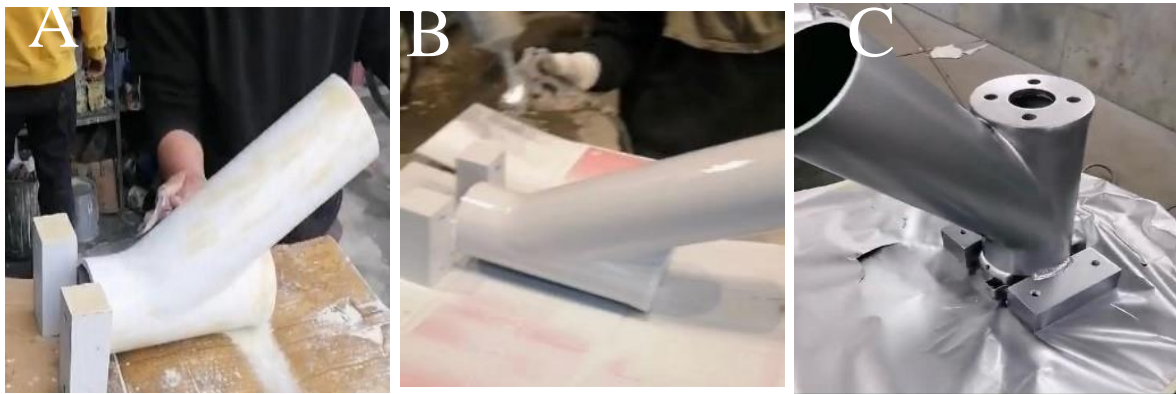
Figure 21: (a) the shape after painting bases, (b) the shape after sanding, and (c) the final shape after the painting was dried via entering the machine into the oven
