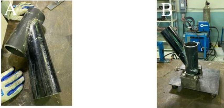
Figure 20: (a) Grinding before welding, and (b) the final shape after the whole welding process is complete
