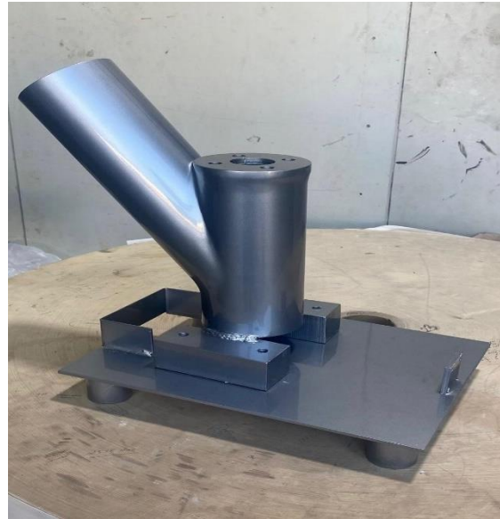
Figure 22: Eco Press: pneumatic cylinder waste crusher
