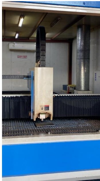
Figure 14: The laser cutting machine and the plate between the piston and the pipe
