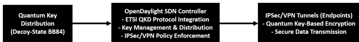
Figure 3: Architecture of the QKD-Integrated OpenDaylight SDN Controller
