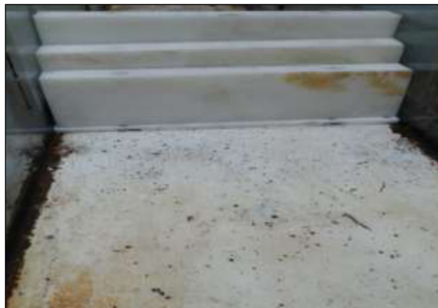
Figure (7): photo of three rectangular vertical submerged breakwaters with different heights back to back
