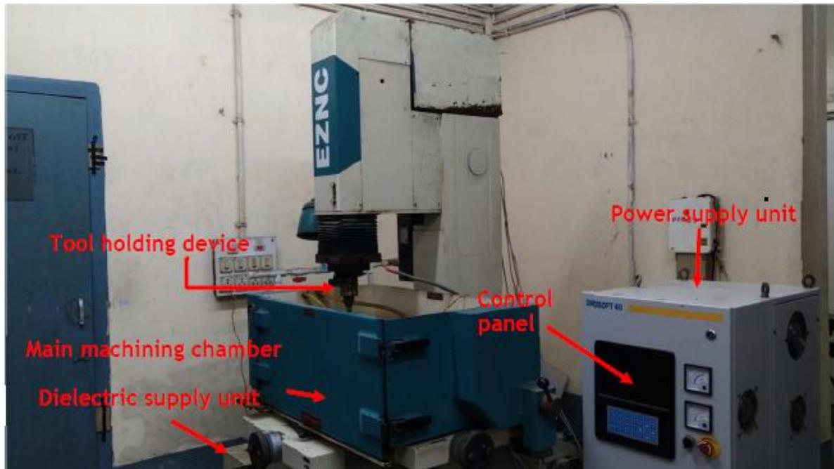
**Fig. 1 Photographic view of S-40 ZNC Die-Sinking EDM Machine**
