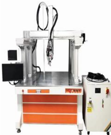
Figure 4: Automatic laser welding
