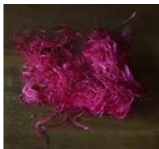
Hydrolyzed reactive dyed nylon yarn
