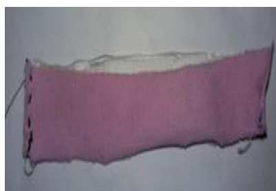
Hydrolyzed reactive dyed fabric after washing
