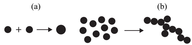
Figure 5. Schematic showing (a) Coalescence; (b) Agglomeration processes.
