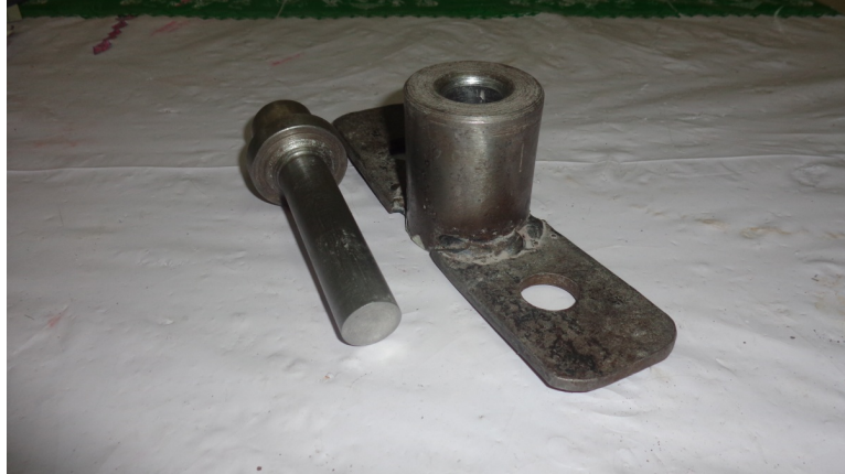
Figure 1 Die set used to fabricate cylindrical preform (see online version for colours)
