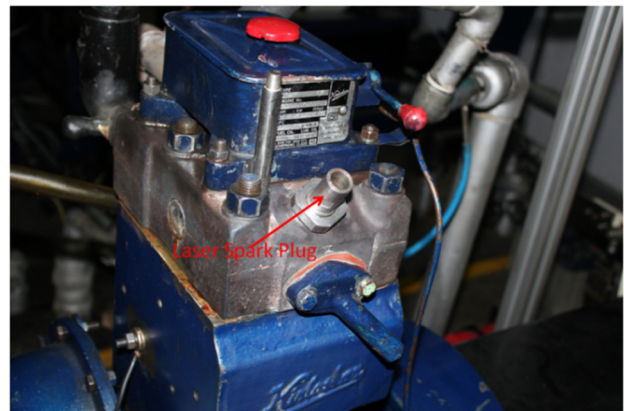
Fig. 2 Laser spark plug installed in the cylinder head.
