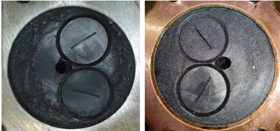
Fig. 11. Carbon deposits on the cylinder head of the engine (a) using EGR (b) without EGR.
