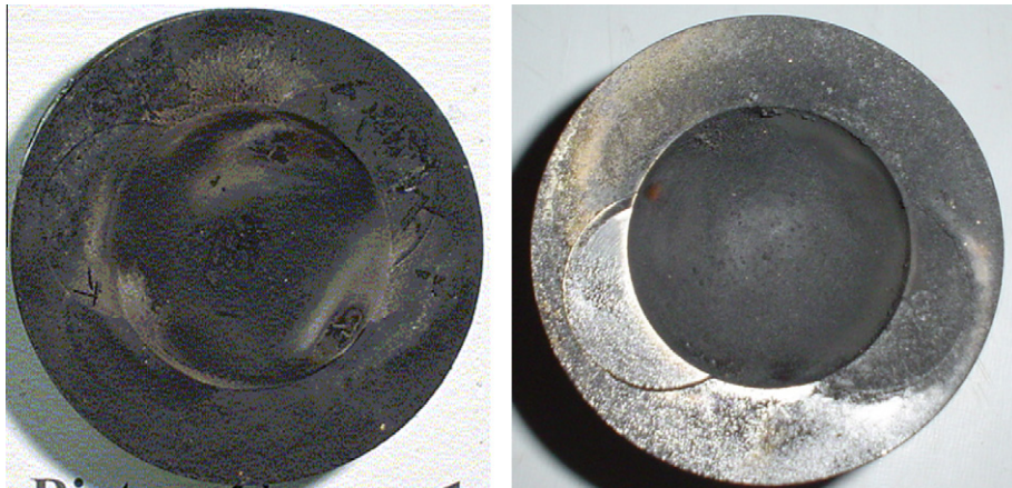
Fig. 13. Carbon deposits on the piston crown of the engine (a) using EGR (b) without EGR.
