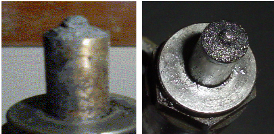
Fig. 12. Carbon deposits on the injector tip of the engine (a) using EGR (b) without EGR.
