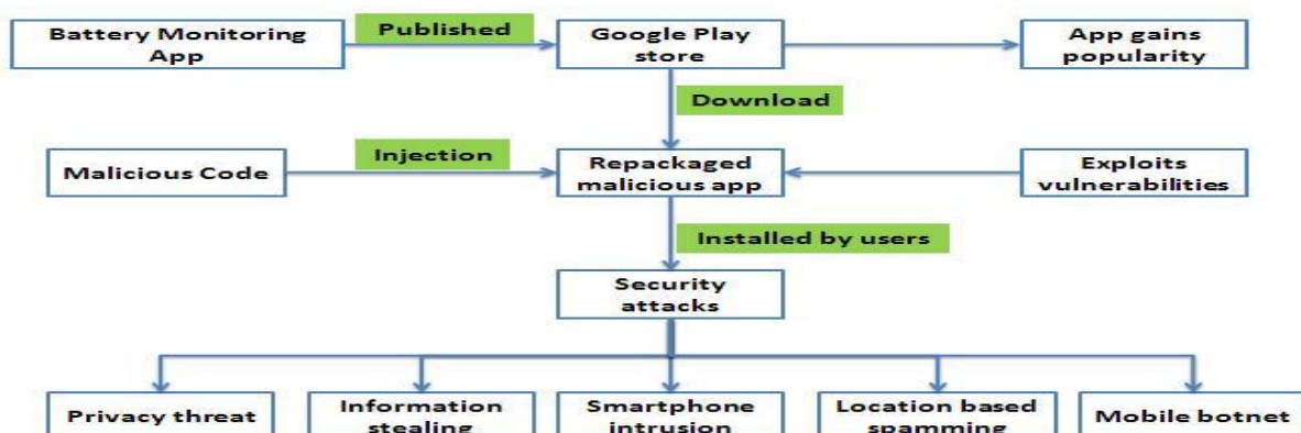
Figure 3: Privacy threat and security attacks based on usage pattern of smartphone and tablet users [14].
