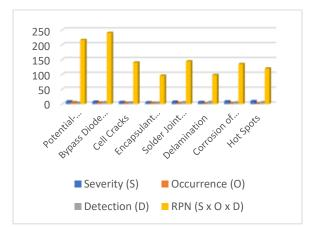
• Potential-Induced Degradation (PID) has a high severity (9), moderate occurrence (6), and detection rating (4), leading to an RPN of 216. This is one of the toppriority failure modes due to its significant impact on system performance.
