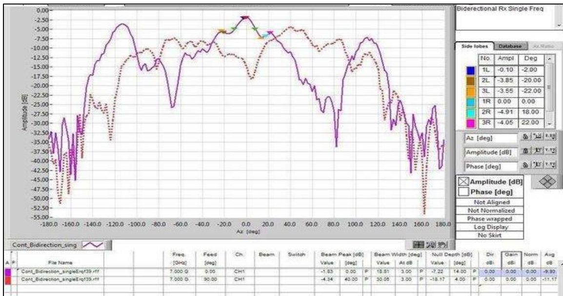
Fig.6. Radiation pattern at 7 GHz
