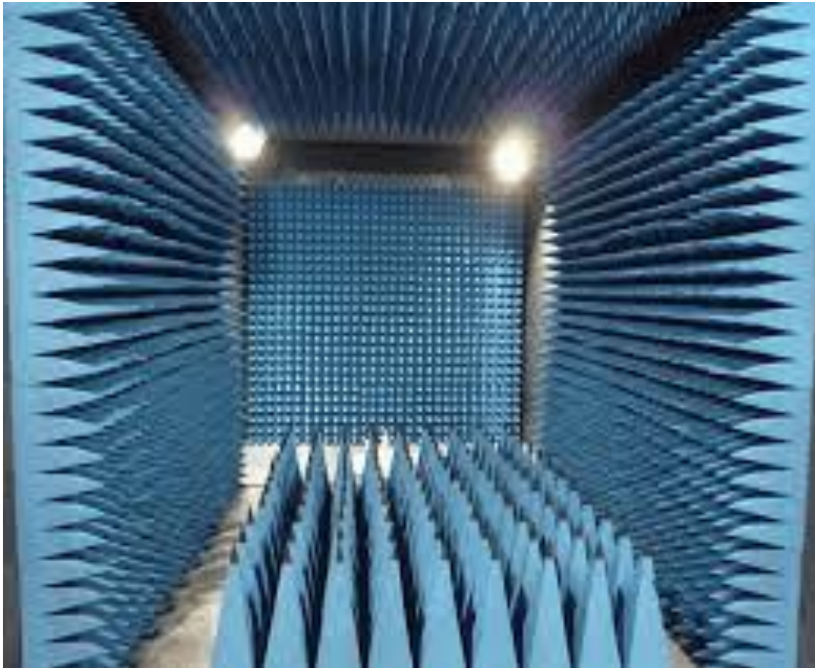
Fig.2 a: Anechoic Chamber for antenna
