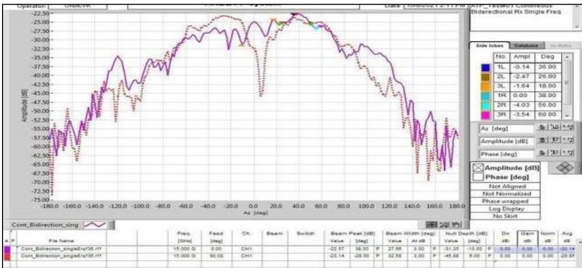
Fig.9. Radiation pattern (Cartesian coordinate system) at 15 GHz
