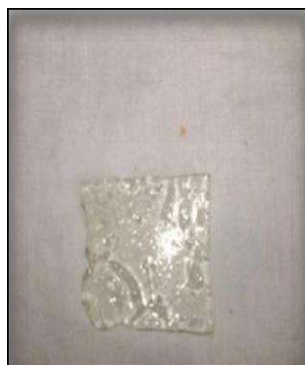
Figure 7 (b). Integrity of PG-3 film at pH 9.2.
