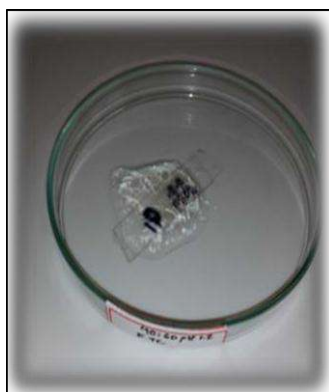
Figure 5 (b). Integrity of PG-3 film at pH 1.2.
