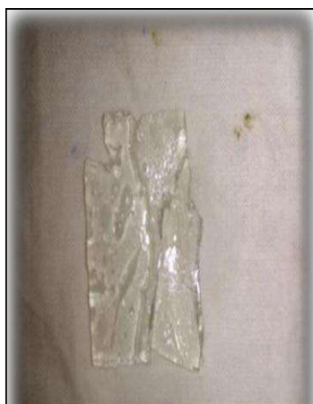
Figure 6 (b). Integrity of PG-3 film at pH 7.4.
