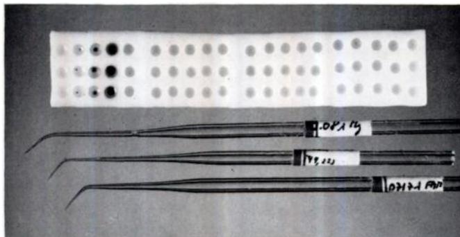
Fig. 1. Teflon oil well rack and constriction pipettes. The scale can be judged by the length of the rack (12 cm). Several of the wells are filled with oil and some contain droplets of three sizes 0.07, 1.3 and 9.1  $\mu$ l, which have been colored for better visualization. These were introduced into the wells with the pipettes shown below the rack.
