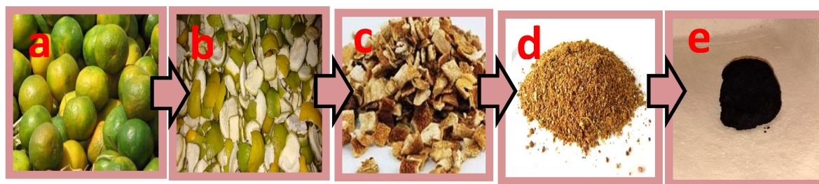
Figure 1. Optical images for the synthesis procedure of SLP-AC (a) Sweet lime (b) Sweet lime peels (c) Dried sweet lime peels (d) Grinded peels (e) SLP-AC after carbonization.
