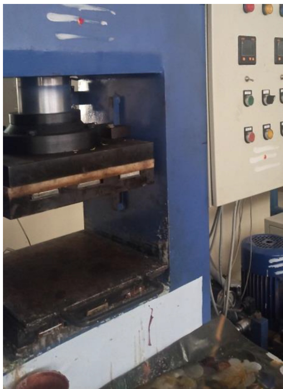
Fig. 2. Compression molding machine used for composite fabrication.
