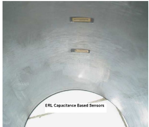
Fig. 3. Liner installed with capacitive micro-sensors.
