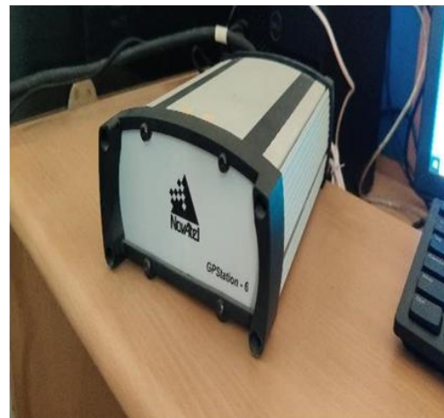
Figure 4. Clear view of Novatel GPStation-6 receiver
