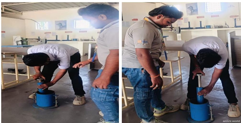
Fig.5: Conducting Compaction factor test for soil mixes
