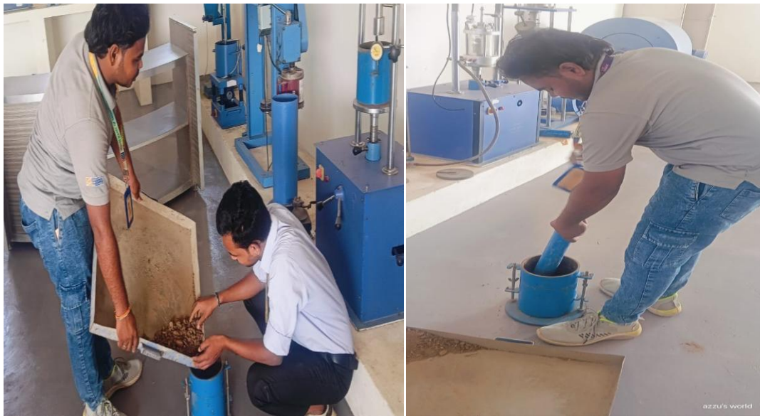
Fig.4: Conducting Standard proctor test for soil samples
