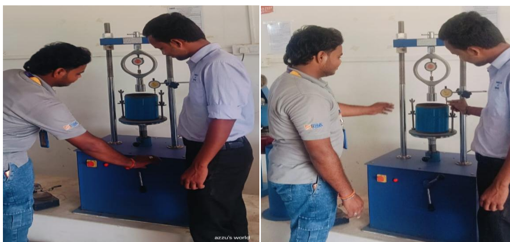
Fig.6: Conducting CBR test for soil mixes
