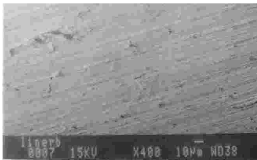
Figure 18: SEM Micrograph of the Liner Surface After 30 Hours at BDC Location
