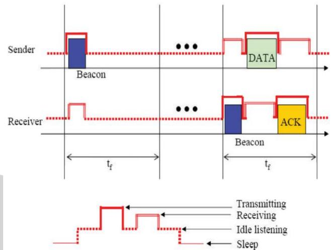
Figure 3.1: Data exchange in 802.11 in ad-hoc mode
