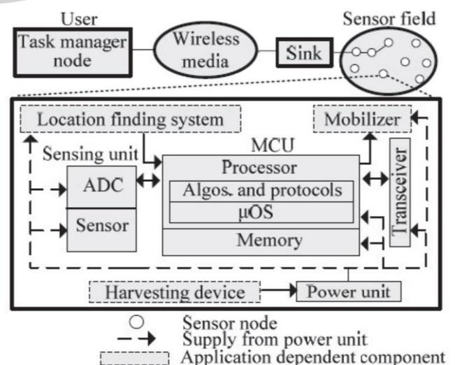
Figure1: WSN design and organization of components of a sensor node.
