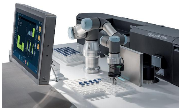
Fig. 2: Robotic pill dispensing is an automation technology used in pharmaceutical plants
