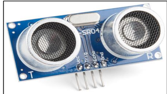
Fig4.9: HC SR 04 Ultrasonic distance sensor
