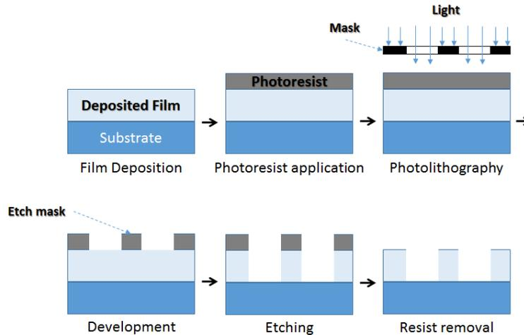
Figure 1. The etching process for wafer fabrication
