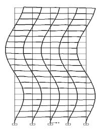
Fig. B.3: Third mode shape of R-20-4 building model
