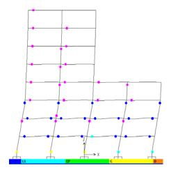
Fig. B.14: Distribution of hinges in S2-8-4 model by uniform load pattern
