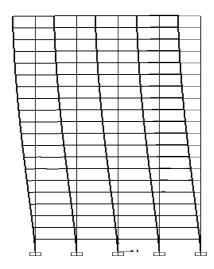
**Fig. B.1**: First mode shape of R-20-4 building model
