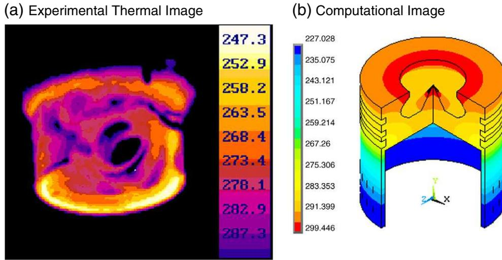
Fig. 2. Steady state temperature distribution for piston geometry with oil jet cooling ( $q'' = 40 \text{ kW/m}^2$ ).
