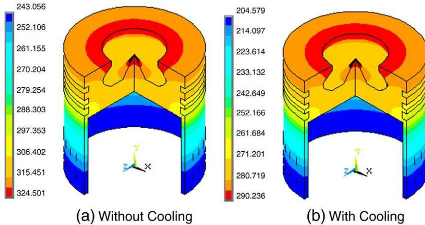
Fig. 3. Steady state temperature profile of the piston without/with oil jet cooling ( $q'' = 45 \text{ kW/m}^2$ ).
