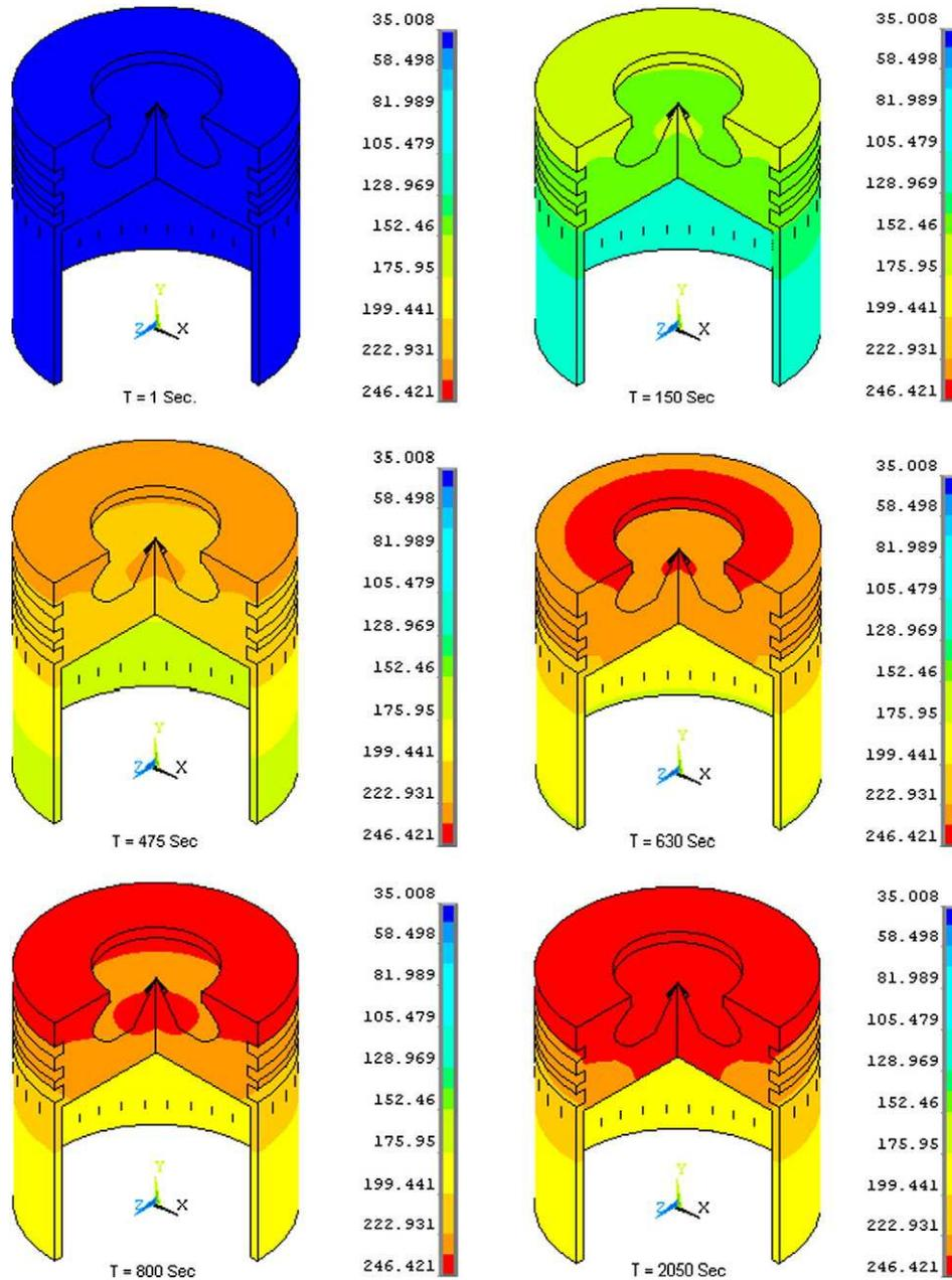
Fig. 5. Transient piston temperatures ( $q'' = 35 \text{ kW/m}^2$ ).
