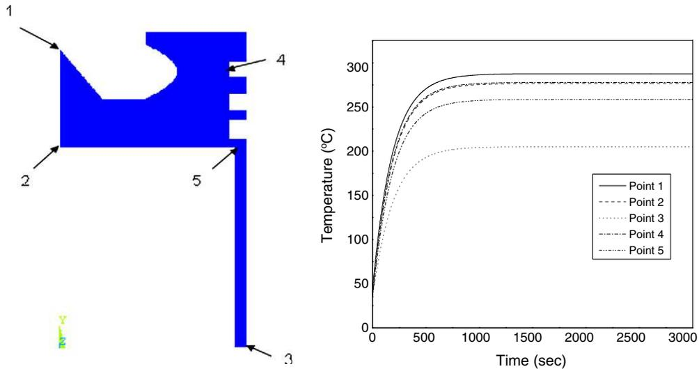
Fig. 4. Piston temperature variation with time ( $q'' = 45 \text{ kW/m}^2$ ).
