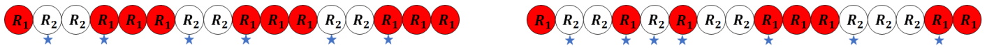
Fig. 2. Mixed-recipe process with fixed-drift (left) and random-drift (right) for the system with two recipes. The star under each recipe shows the communication hop at the run of changing recipe.
